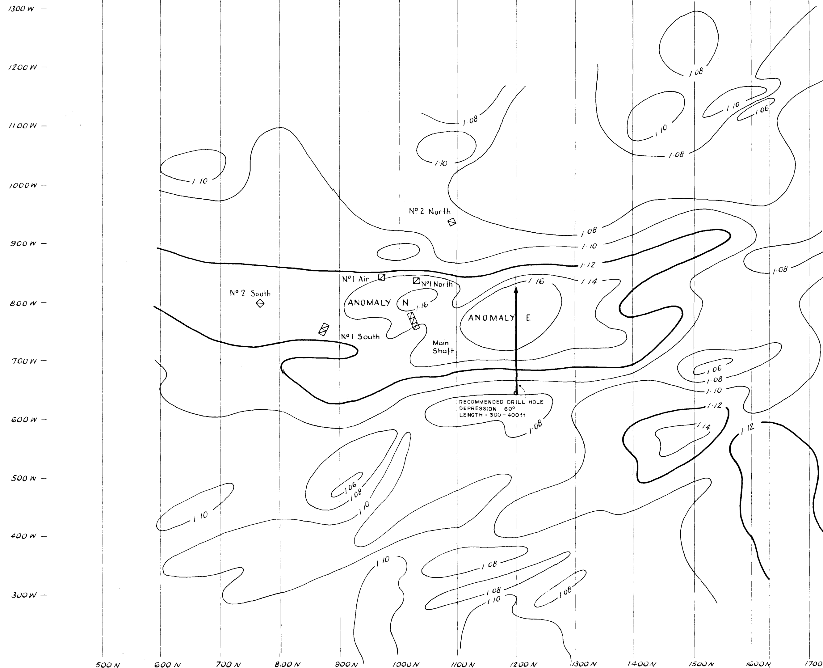
TURAM RATIO CONTOURS IRON BLOW MINE, NT GEOPHYSICAL SURVEY, NOVEMBER 1960.
